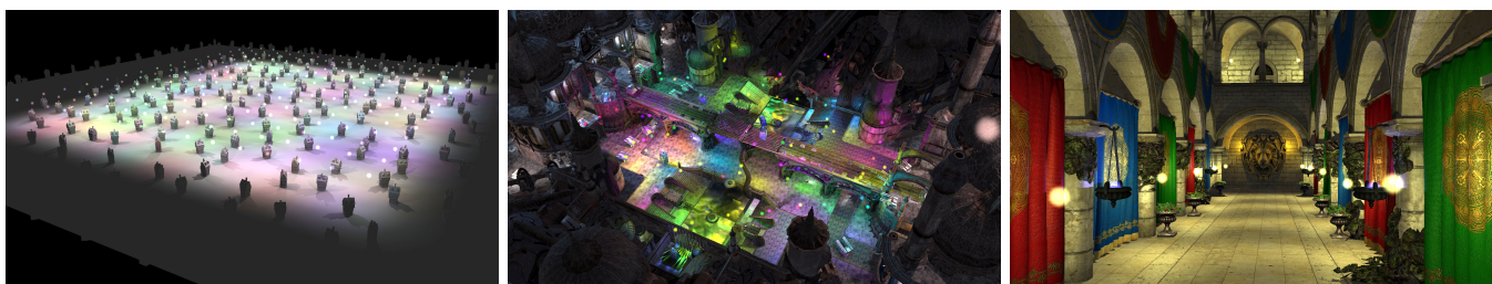
Fig. 1. Scenes rendered with many lights casting shadows at 1920 \times 1080 resolution on an NVIDIA Geforce Titan. From the left: HOUSES with 1.01M triangles and 256 lights (23ms), NECROPOLIS with 2.58M triangles and 356 lights (34ms), CRYSPONZA with 302K triangles and 65 lights (16ms).
